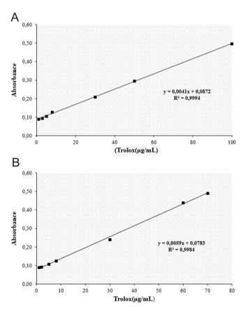
Figure 4. Trolox standard graph. A. Ethanol. B. Methanol.
