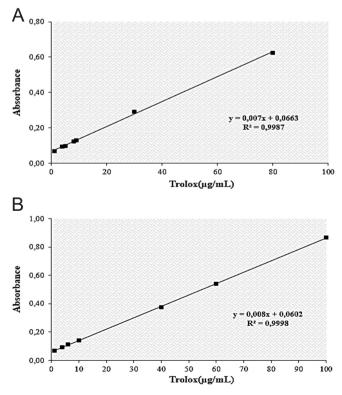
Figure 3. Trolox standard graph. A. Ethanol. B. Methanol.
