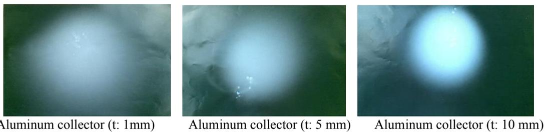
**Figure 2.** Collection area of the nanofibers obtained with circular aluminum collectors of different thicknesses.
