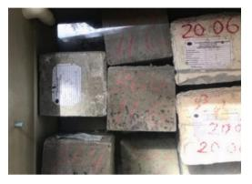
Figure 4. Curing of samples in curing pool
