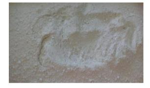
Figure 1. Marble powder used in the production of SCLWC samples
