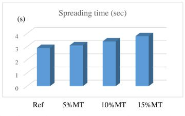
Figure 6. Spread time (T500 time) test results of SCLWC samples
