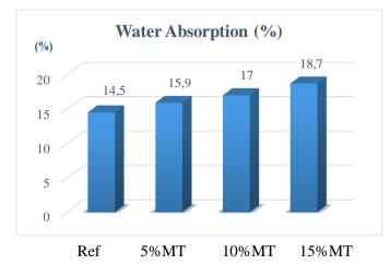
Figure 10. Water absorption test results of SCLWC samples
