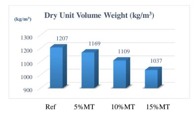
Figure 11. Dry unit volume weight test results of SCLWC samples
