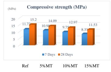
Figure 12. Compressive strength test results of SCLWC samples
