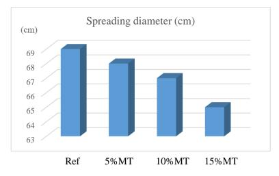
Figure 5. Slump-dispersion test results of SCLWC samples
