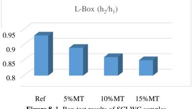
Figure 8. L-Box test results of SCLWC samples
