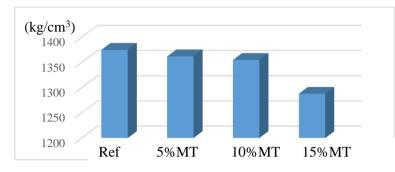
Figure 9. Fresh concrete UVW test results of SCLWC samples
