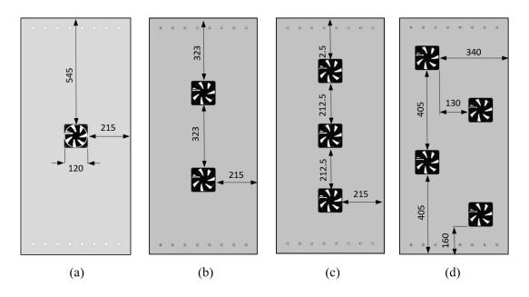
**Figure 3.** Layout plans of DC fans placed behind the PV panel (a) with 1 DC fan (b) with 2 DC fan (c) with 3 DC fan and (d) with 4 DC fan
