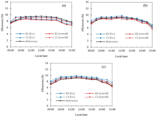
Figure 5. Efficiency values of PV panels with 1 and 2 DC fans
