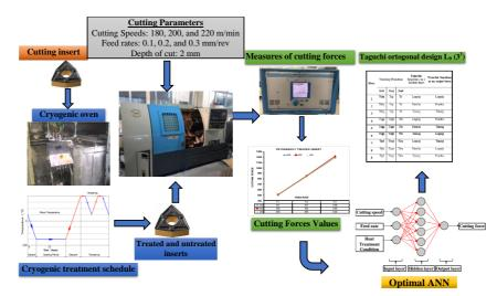
Figure 2. Schematic representation of ANN and experimental setup
