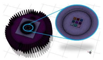
Figure 2. Mesh model of the COB LED and heat sink domains.
