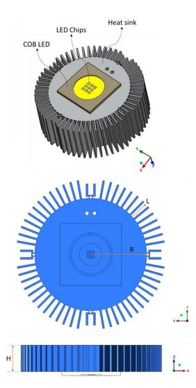
Figure 1. COB LED and heat sink model with optimization parameters.
