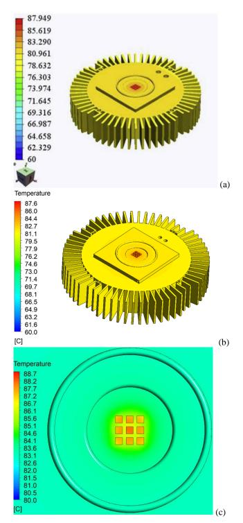
**Figure 3.** Temperature distributions of COB LED and heat sink presented by a) Wu et al. [14], b) this study, and c) COB LED detail in the present study.
