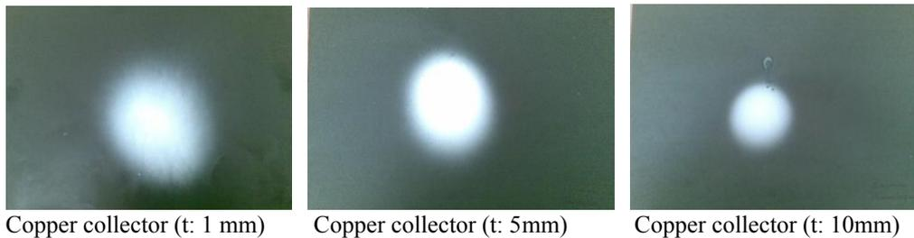
**Figure 3.** Collection area of the nanofibers obtained with circular copper collectors of different thicknesses.
