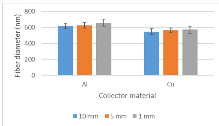
**Figure 4.** Average diameter values of nanofibers obtained with circular aluminum and copper collectors.
