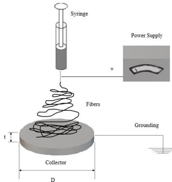
**Figure 1.** The schematic view of electrospinning setup used in this work.
