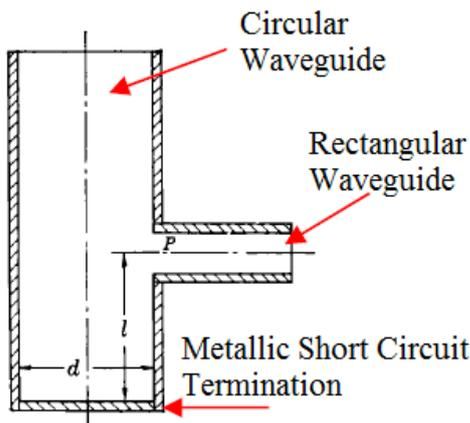
Figure 1. Rectangular-to-circular waveguide structure [20].
