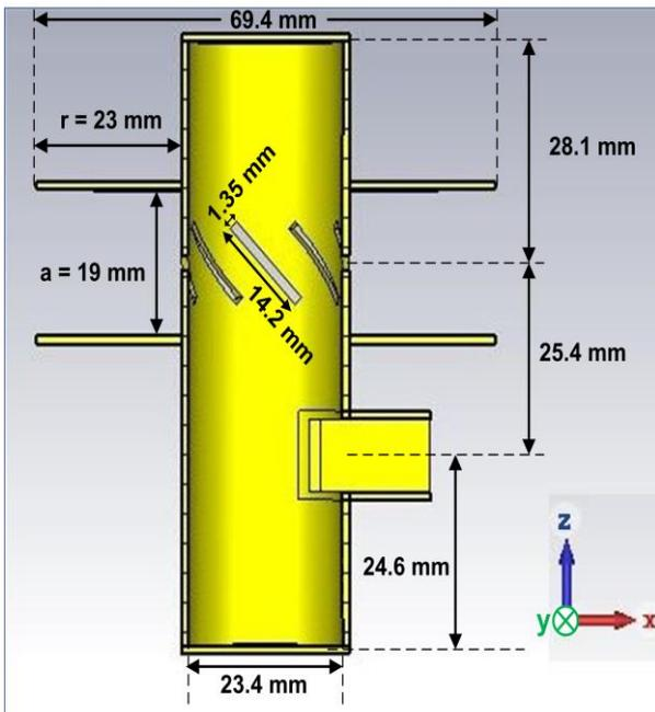
**Figure 11.** The dimensions of the designed antenna with identical slots for telemetry purpose (transmitter structure).
