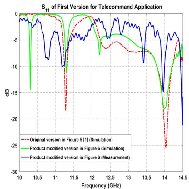
**Figure 7.** The magnitude of reflection coefficient ( $S_{11}$ ) of the designed receiver antenna.
