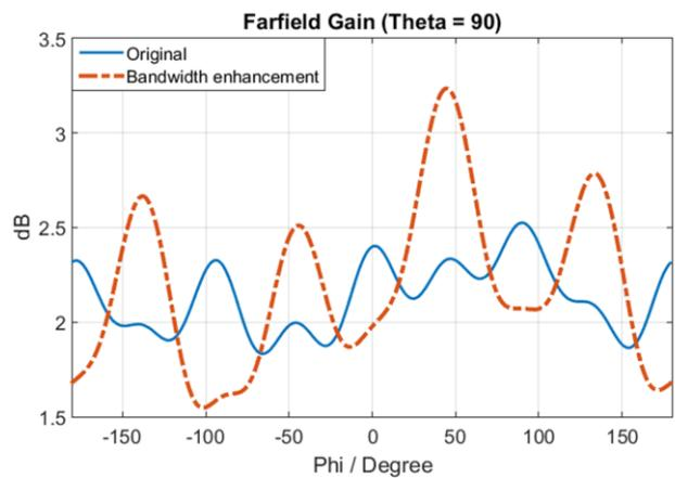
**Figure 13.** Rectangular radiation patterns of the antennas of first and second versions in azimuth plane at 11.75 GHz.
