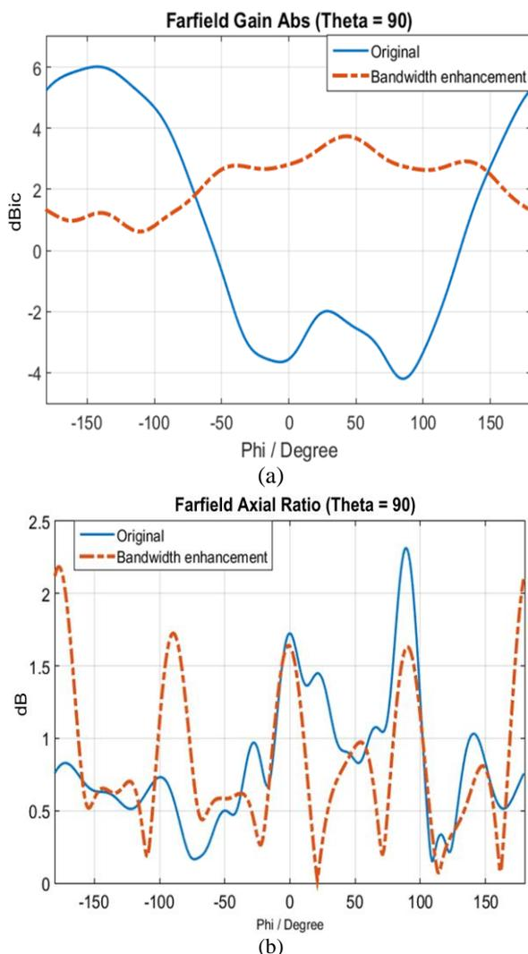
**Figure 15.** (a) Rectangular radiation patterns and (b) axial ratio of the antennas of first and second versions in azimuth plane at 12.25 GHz.
