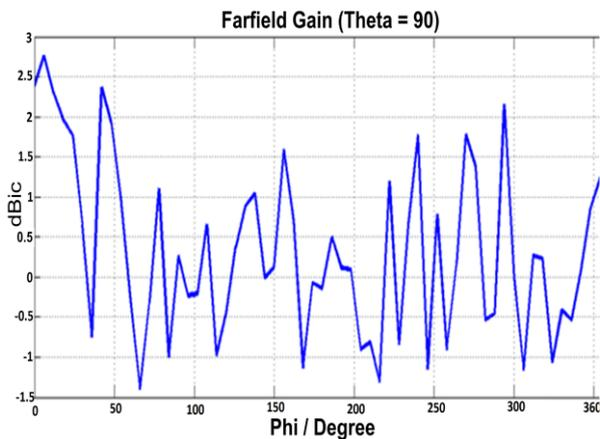
**Figure 9.** Measured rectangular gain pattern at the azimuth plane for receiver (telecommand) antenna at 14 GHz.
