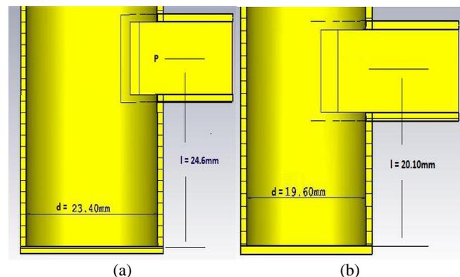
Figure 2. Final dimensions belonging to designed rectangular-to-circular waveguide transition (a) for transmitter structure (b) for receiver structure.
