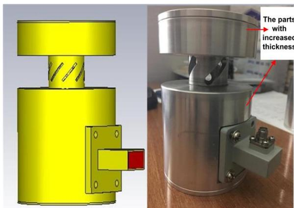
**Figure 6.** The simulation view and photograph of the manufactured receiver antenna.
