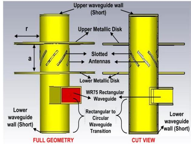
**Figure 4.** The proposed circularly polarized omnidirectional antenna structure along with cut view for both versions.
