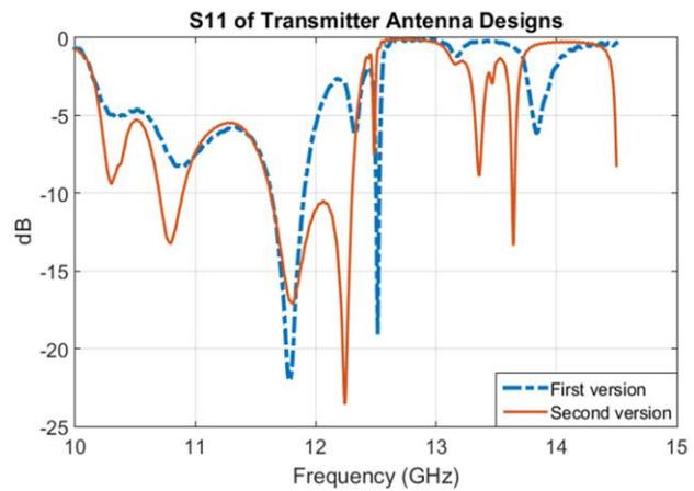
**Figure 12.** The magnitude of reflection coefficient ( $S_{11}$ ) of the designed transmitter (telemetry) antennas.
