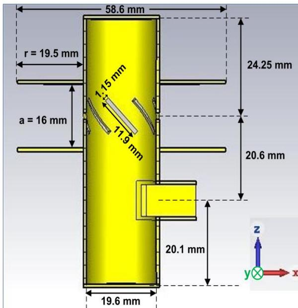
**Figure 5.** The simulation view of the designed antenna for receiver structure.
